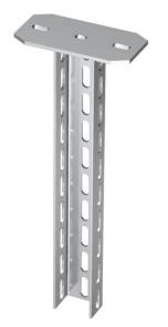
Suspended support (U profile) with welded head plate. For fastening to horizontal concrete ceilings and steel girders. For bracket widths of 400 mm or more, or if the bracket is mounted at the end of a suspended support, we recommend the use of the spacer, type DSK 61.
