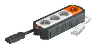
The ready-for-connection UTC4 universal support has 3 pre-installed 33° protective contact sockets in white and one pre-installed 33° protective contact socket in orange, 250 V~, 16 A. With halogen-free connection cable. Suitable for VL connection cables and device installation units of nominal size R7, R9 and 9.
