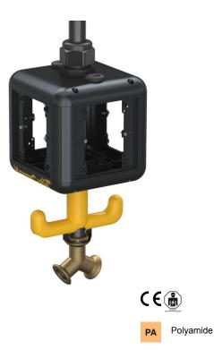
Empty housing with 1 m pipe 1/2" and connection for compressed air hose 13 x 3.5 mm and 2-way distributor 1/2". With suspension lug and grip hook, for the installation of four electrical resources, with included partition. Without cover plates.
