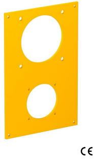
Cover plate with a Ø 45 mm opening for the installation of one extension socket (type ASD-...) with 38 mm fastening track and a Ø 60 mm opening for the installation of one CEE socket 16/32 A with 60 mm fastening track, including 8 screws for fastening the device.
