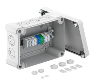
Junction box for the connection of cables and lines indoors and in outdoor areas. Rectangular design with knock-out entries. Suitable for wall and ceiling mounting with the option to fasten outside, inside or to mount via the corner domes. Particularly impact resistant with IK09. Cover with quick lock, sealable. Made from halogen-free and UV-resistant materials.
