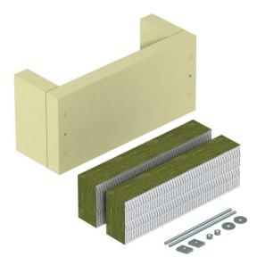
Strain relief as an effective support measure for vertical cable routing, according to DIN 4102 Part 12, approved for all cable types and all vertical routing systems. Maintenance of electrical function classes E30 to E90. Housing including mineral fibre panels, fastening material, ASX fire protection coating in cartridge and identification plate.
