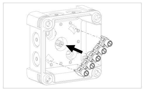
Figure 10: Insert the terminal strip, type 689, in the junction box
