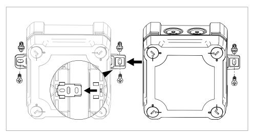
Figure 20: Connecting junction boxes with the fastening strap
