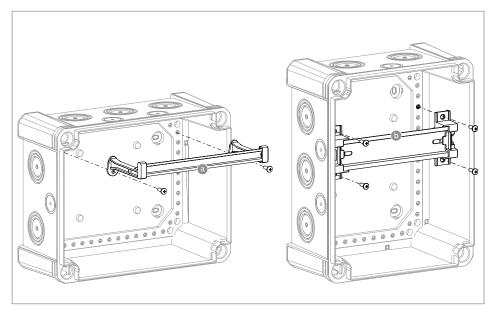
**Figure 14:** Mount the hat profile rail, type 46277 A and type 2069 B , in the junction box
