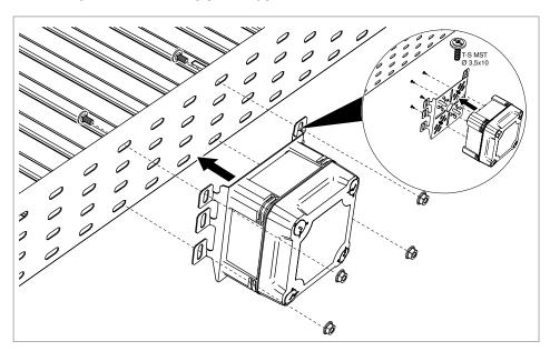
Figure 23: Mounting the junction box on cable trays
