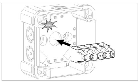
Figure 11: Insert the terminal strip, type KL-T 02-06, in the junction box
