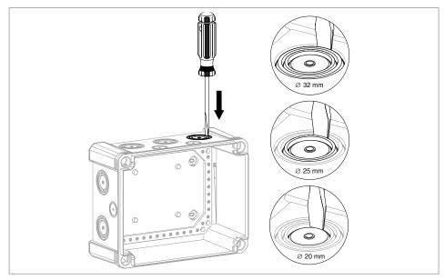
Figure 5: Opening a knockout entry
