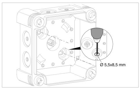
Figure 16: Drilling holes in the rear panel
