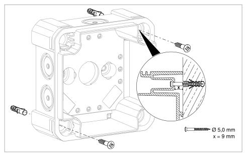
Figure 18: Screwing the junction box to the wall through corner holes
