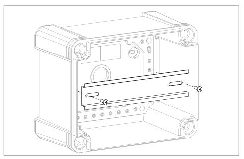
Figure 12: Inserting the hat profile, type 2069, without a support in the junction box
