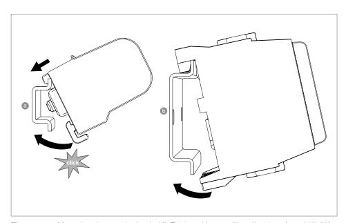
**Figure 15:** Mounting the terminal strip KL-T 06 and hat profile rail 46277 A and HLAK on hat profile rail 2069 B
