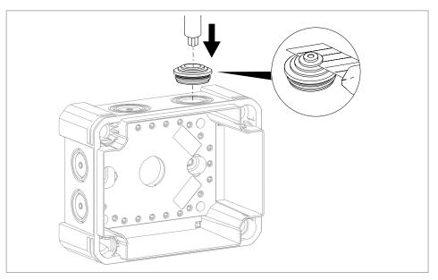
Figure 9: Stepped cutting of the plug-in seal
