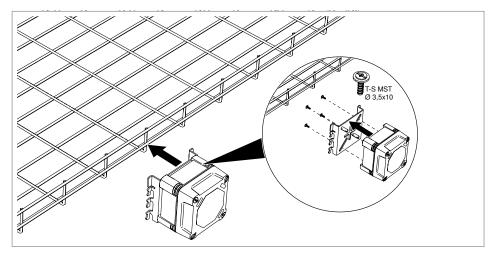
Figure 21: Mounting the junction box on mesh cable trays
