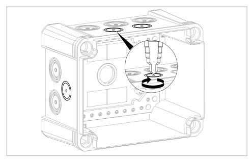
Figure 6: Drilling a hole in the pre-marking
