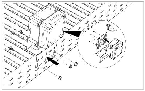
Figure 22: Mounting the junction box on cable trays
