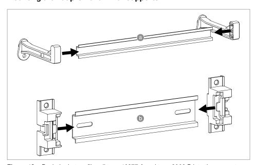
Figure 13: Push the hat profile rail type 46277 A and type 2069 B into the support
