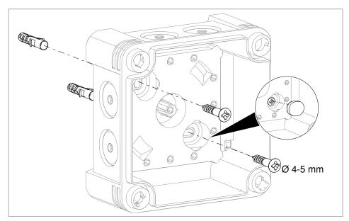
Figure 17: Screwing the junction box to the wall
