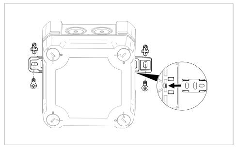
Figure 19: Mounting the junction box on the wall using the fastening strap
